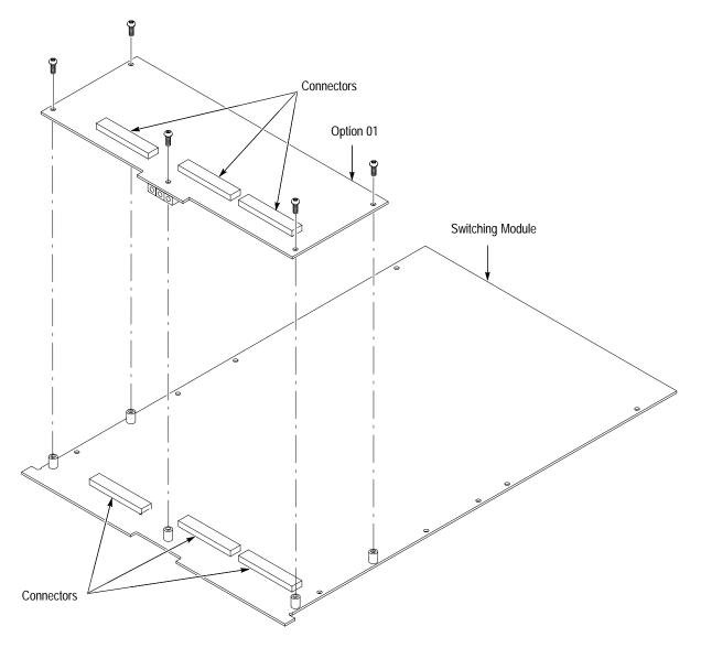
Figure 1–3: Mounting the Option 01
